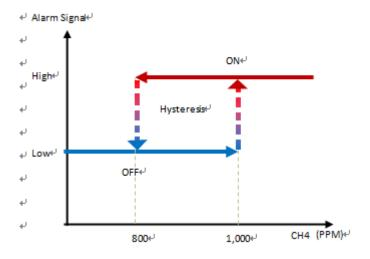
EK-100SL series is available for customer to enable to change alarm activation & deactivation point.
