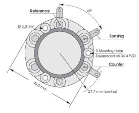
All dimensions in mm All tolerances ±0.15 mm unless otherwise stated 3NT shown with side tags and tin pins
