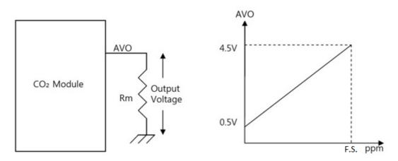
Measured Voltage 0.5V~3.0V match proportionally to 0~5,000 ppm .
