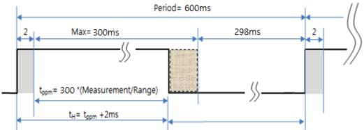
EX) t<sub>H</sub> (High Pulse Width) calculation for 50 ppm in 100 ppm Reading Range.
