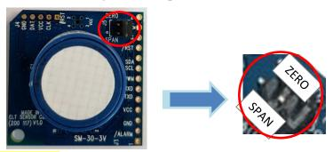
Normal mode-#1 is for mobile-H2S-meter or fixed type H2S-meter installed where H2S gas almost ever-present environment.
