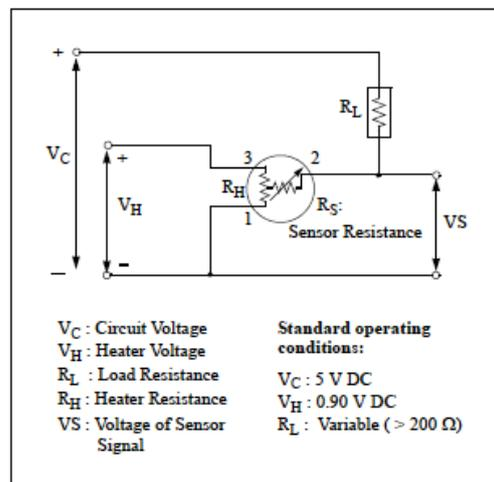
Fig 2. Standard circuit
