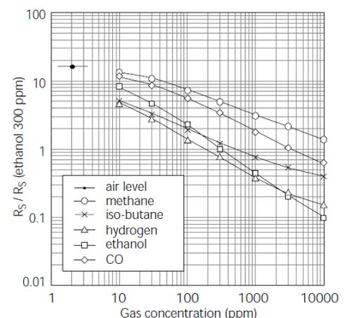
Fig3. Sensitivity characteristics
