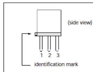
Fig 1c. Pin Layout
