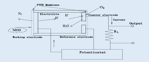
The NE4-NH3-5000 consists of 3 porous noble metal electrodes separated by an acidic aqueous electrolyte, housed within a plastic (PPO) enclosure. Gas enters the cell via a gas phase diffusion barrier. An electrolyte reservoir ensures an excess of electrolyte is available at all times, and the sensor is vented to ensure that the internal and external pressure of the sensor is always in equilibrium.
