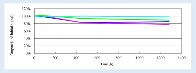
**Low Temperature:** The following graph illustrates the signal output stability for a sensor exposed to -20°C over 10,000 hours. The NH<sub>3</sub> concentration used was 10ppm NH<sub>3</sub> in air.
