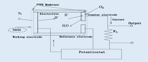
The NE4-NH3-1000 consists of 3 porous noble metal electrodes separated by an acidic aqueous electrolyte, housed within a plastic (PPO) enclosure. Gas enters the cell via a gas phase diffusion barrier. An electrolyte reservoir ensures an excess of electrolyte is available at all times, and the sensor is vented to ensure that the internal and external pressure of the sensor is always in equilibrium.
