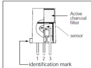
Fig 1c. Pin Layout
