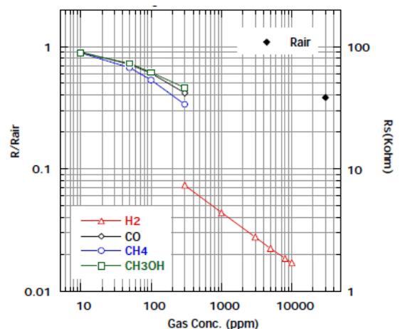
Fig 3. Sensitivity characteristics
