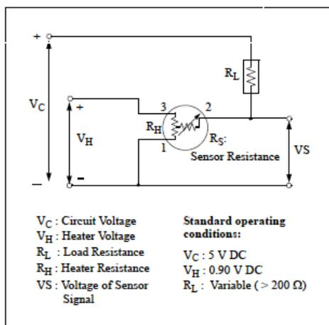
Fig 2. Standard circuit
