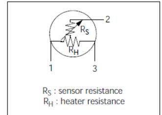
Fig 1d. Equivalent circuit
