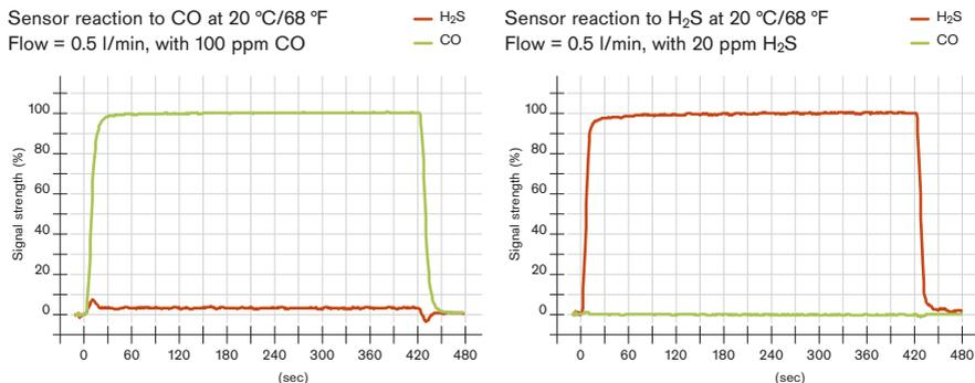
The values shown in the following table are standard and apply to new sensors. The values may fluctuate by  $\pm 30\%$ . The sensor may also be sensitive to additional gases (for more information, please contact Dräger). Gas mixtures may be displayed as the sum of all components. Gases with a negative cross sensitivity may displace an existing concentration of CO or H<sub>2</sub>S. To be sure, please check if gas mixtures are present.
