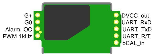
Figure 2. Pin assignment
