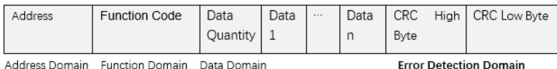
Frame delimitation: In Modbus RTU mode, the sending/receiving time interval between each two characters cannot exceed 1.5 times of the character transmission time. If the time interval between two characters exceeds 3.5 times of the character transmission time, it is considered that one frame of data has been received and a new frame of data transmission begins.
