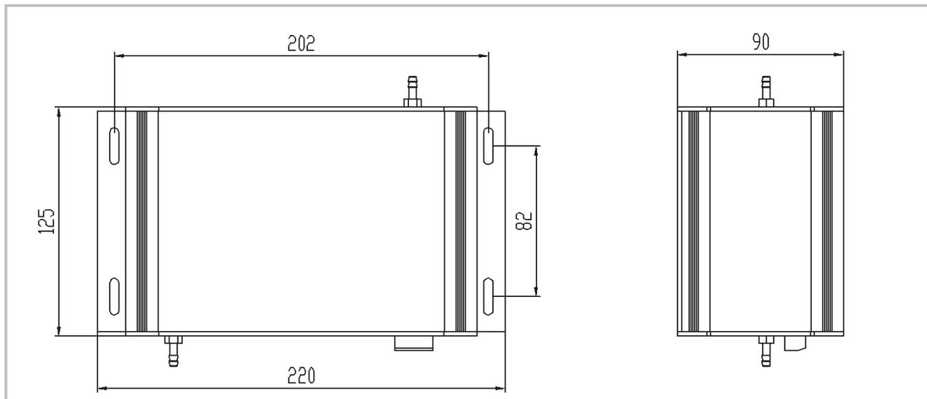
OPM-6303M Structure (Unit: mm; Tolerance:  $\pm 2$  mm)
