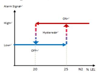
2<sup>nd</sup> Alarm use VoL / VoH TTL signal Switching instead of SPST (Single Pole Single Throw) method. EK-100SL series is available for customer to enable to change alarm activation & deactivation point.
