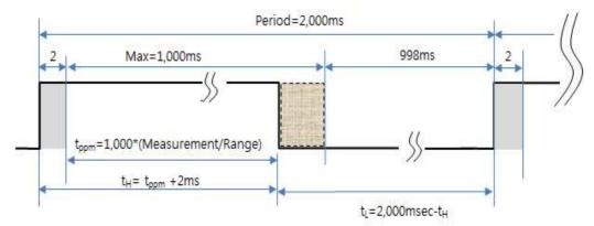
EX) t<sub>H</sub> (High Pulse Width) calculation for 50% LEL in 0~100% LEL Range.
