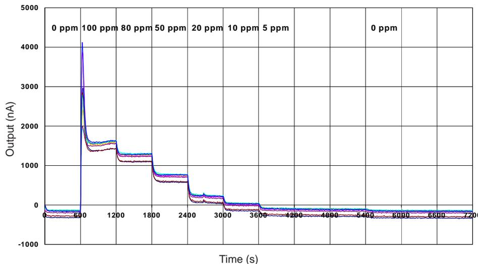
With good sensor response as low as 5 ppm Hydrogen, this sensor can be used for leak detection and process control.
