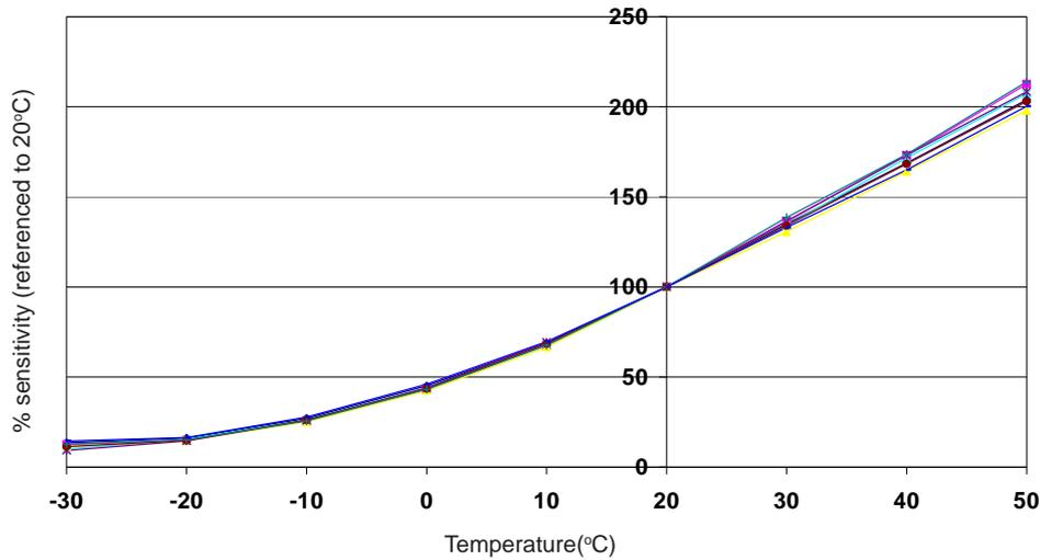
Figure 2 shows temperature dependence of sensitivity to 400ppm Hydrogen.
