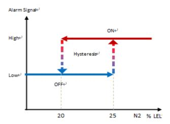
Alarm use Vol / VoH TTL signal Switching instead of SPST (Single Pole Single Throw) method. EK-100SL series is available for customer to enable to change alarm activation & deactivation point.
