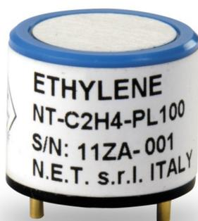
The NT-C2H2-PL100 is a new electrochemical gas sensor with 3 electrodes for the detection of Ethylene in a variety of gas detection applications. Exhibiting high performance with very stable base line and output signal and excellent selectivity, this compact sensor (20.4 mm diameter) is suitable both for portable and fixed gas detection instruments.
